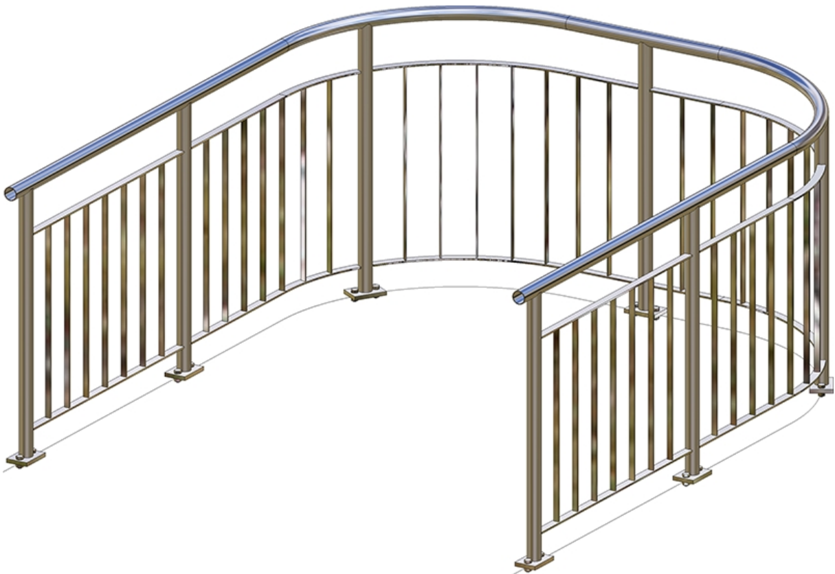
Curved railing, created on the basis of arcs
